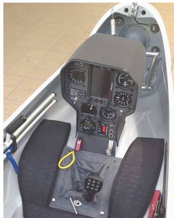
The tall (optional) instrument panel. The yellow ring is the tow cable release
