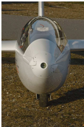
The folded blades lay close to the airframe without touching it.
