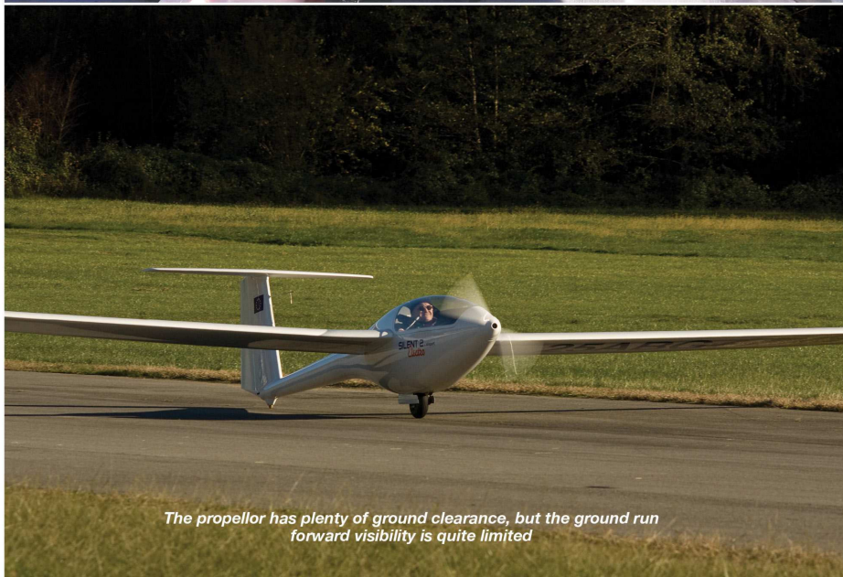
Climbing at a steady 2 m/s, the engine draws 17 kW out of a max of 23 kW at full power. Level flight requires only 4-5 kW of power.
